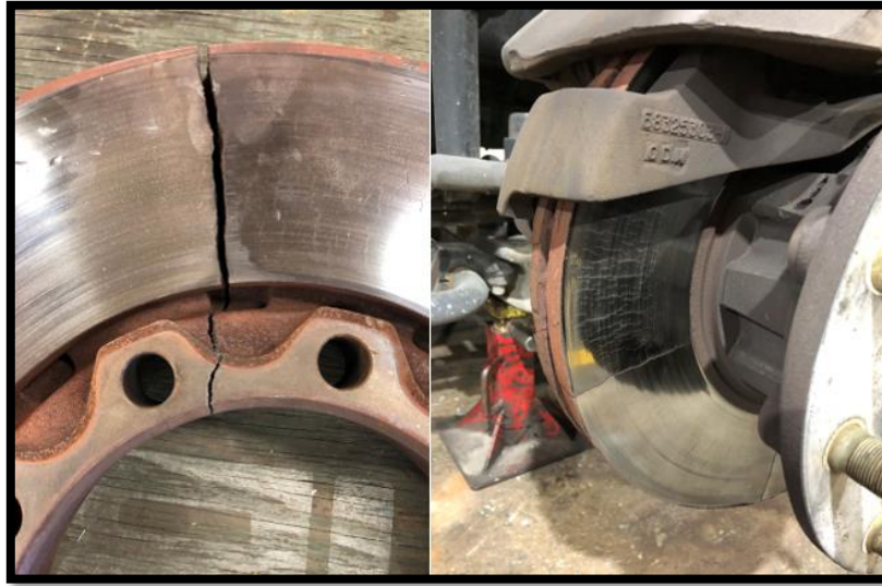
(Example of failed rotors)
