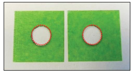
**STEP 8:** Apply the masking tape sections to the area surrounding the mounting surfaces for the propeller shaft center brace bolts on both the left and right sides. Refer to Work Tips Video at 00:30.
