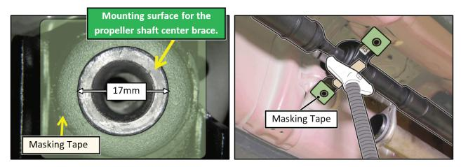
**STEP 9:** Using a 3M Scotch-Brite Hand Pad or 240-320 grit emery cloth, **CAREFULLY** remove the paint on the mounting surface contact area for the left and right propeller shaft center brace bolts. Confirm there is no paint left on the surface when completed.
