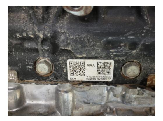
The engine broadcast code can be found on the lower right of the engine block.
