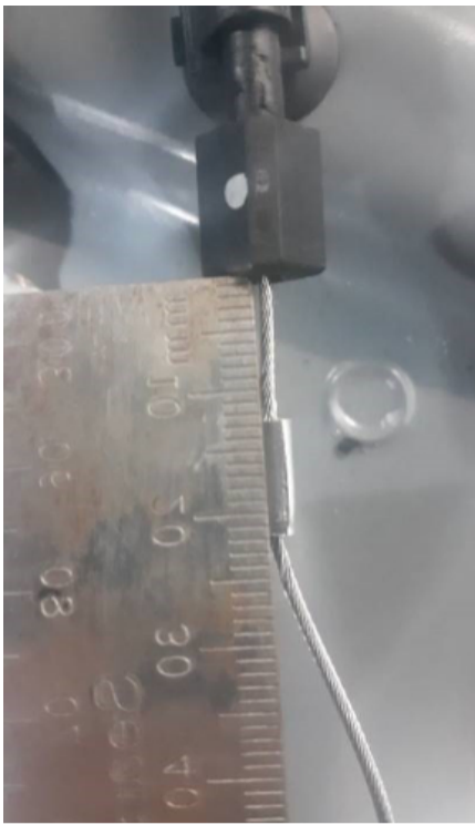
Figure 2 – Proper length for a fully retracted cable (~12 mm).
