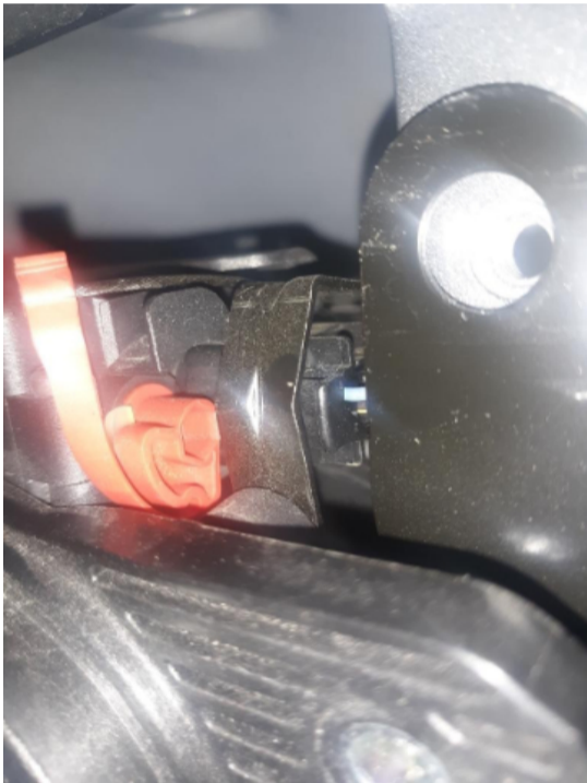
Figure 3 – View at the receptacle end with a cable in an improper position from being pushed.
