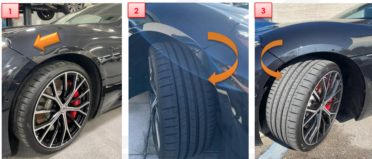
Start with the wheels pointing straight Turn the wheels fully locked to the Right Turn the wheels fully locked to the Left
