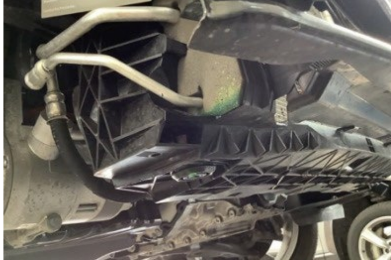
Figure 2. High and low side refrigerant lines routing through the lock carrier.
