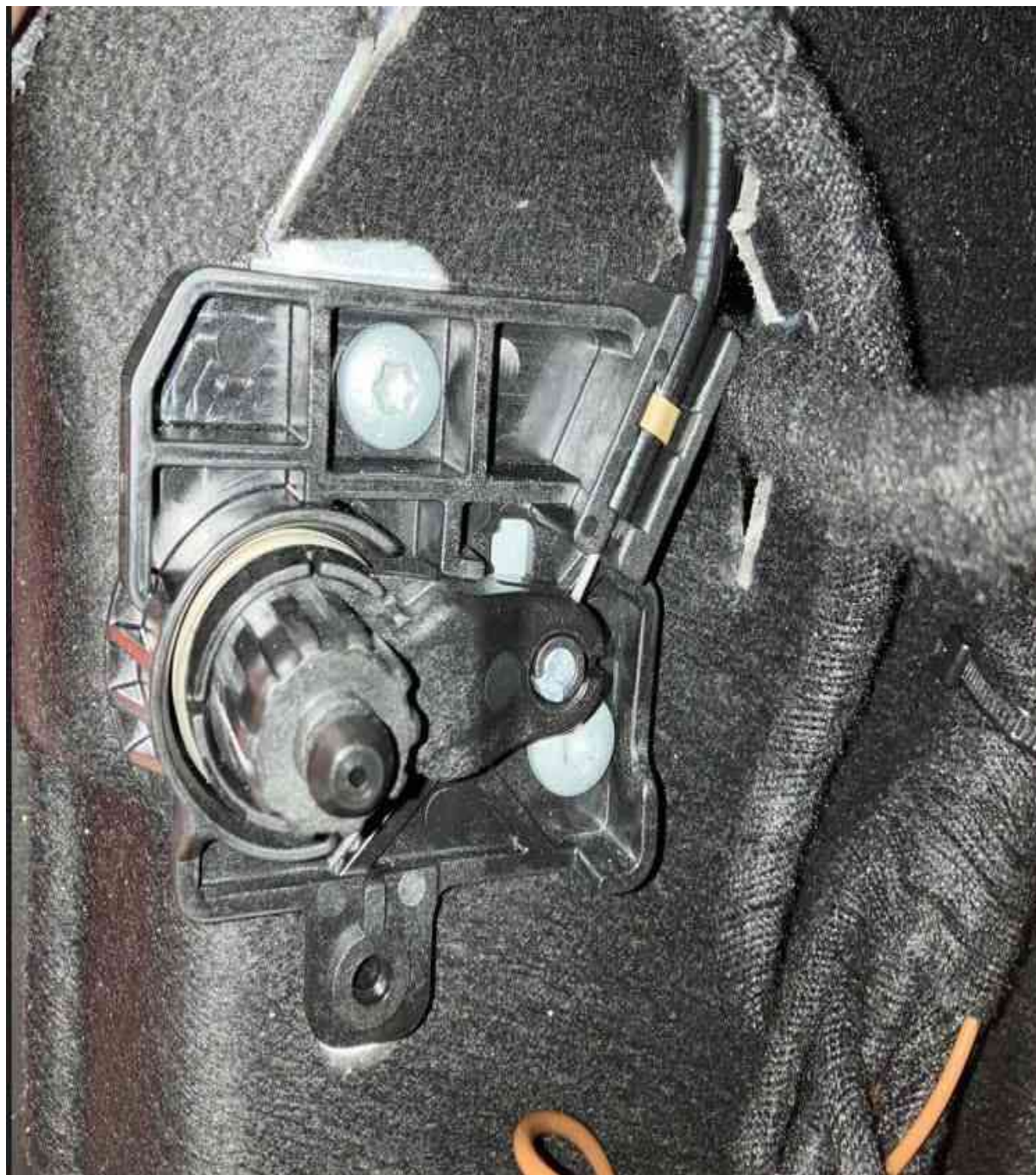
Figure 5. Reinstall the Bowden cable in the mounting bracket after turning the nipple.
