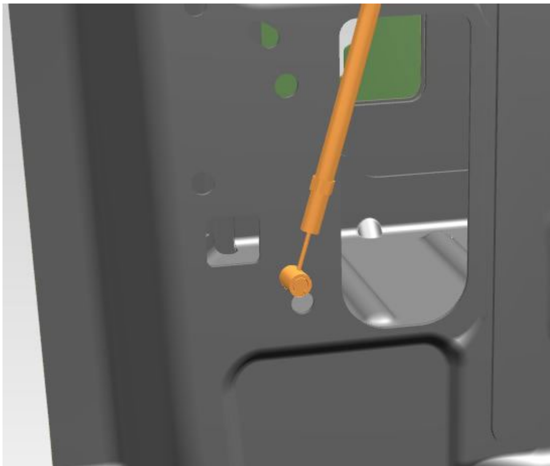
Figure 3. Bowden cable removed from mounting bracket.
