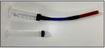
3. Reinstall the syringe plunger and push in the plunger until sealant begins to flow out at the end of the syringe.
