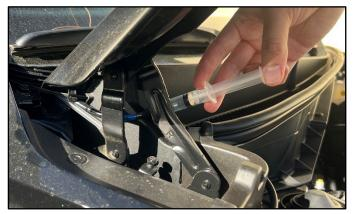
7. Remove the syringe, but leave the barrier tube in place for 10 minutes.
