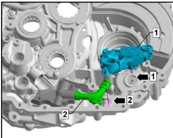
• Install new O-ring <1> from the repair kit on the changeover valve oil pipe.
