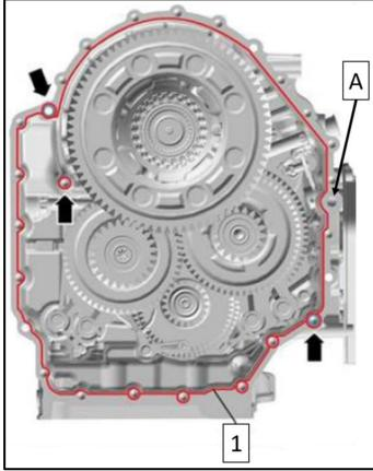
• Install new o-ring <1> from the repair kit.
