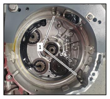
• Alternate view of the two bolts <1> <u>that are</u> <u>not removed</u> at this time.
