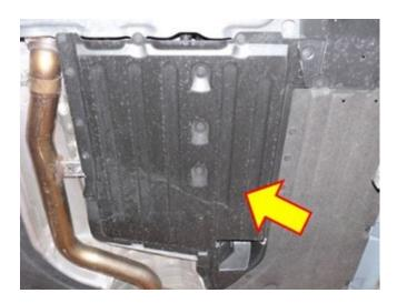
1. Remove the underbody protection panel following the repair instructions listed in AIR/ISTA (51 47 491).
