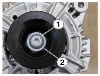
• Check the retaining screw (1) for the hexagon nut (2) on the SGR drive pulley.
