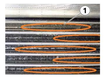
• Example: Belt debris in pulley grooves (1).
