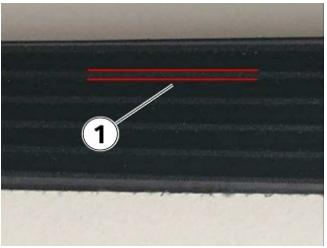
The ribs may be narrower or worn thin (1).
