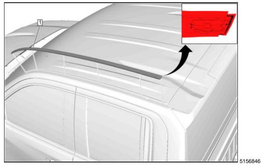
**Note:** Use caution when removing the Passenger Side Roof Panel Joint Finish Molding to prevent damage to either the part or the roof.
