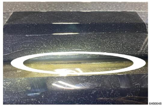
Note: The crack can be located anywhere along the channel and may be difficult to see.
