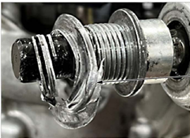
STRIPPED THREADS CAUSED BY EXCESSIVE TORQUE.
