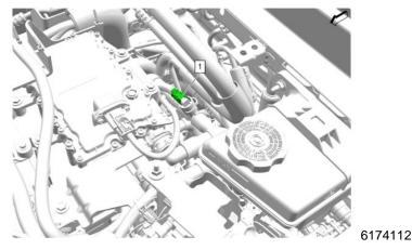
2. Locate the B388B Hybrid/Propulsion System Coolant Temperature Sensor 2 (1).
