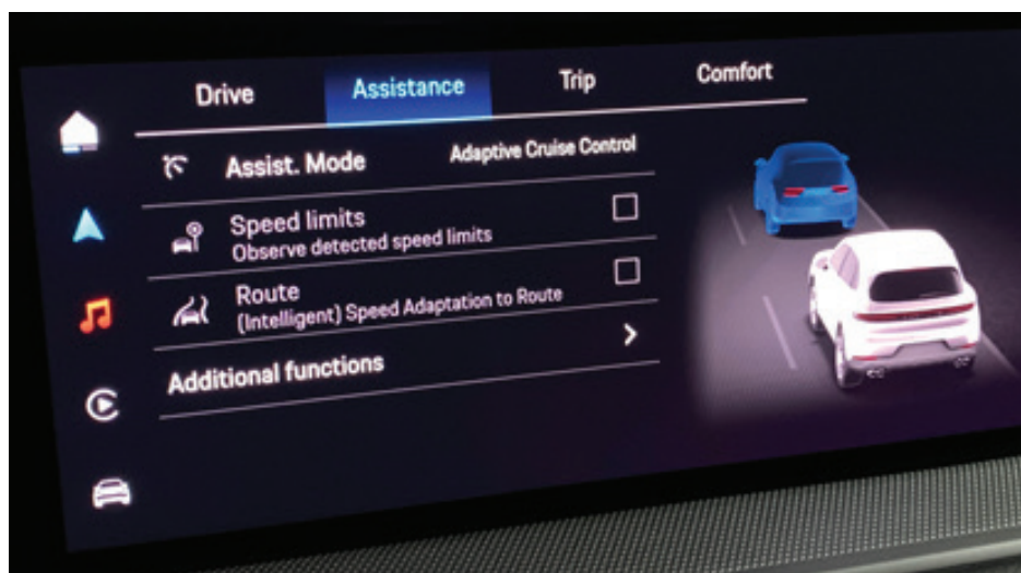
Figure 1- Active Lane Keep Assist function missing from PCM
