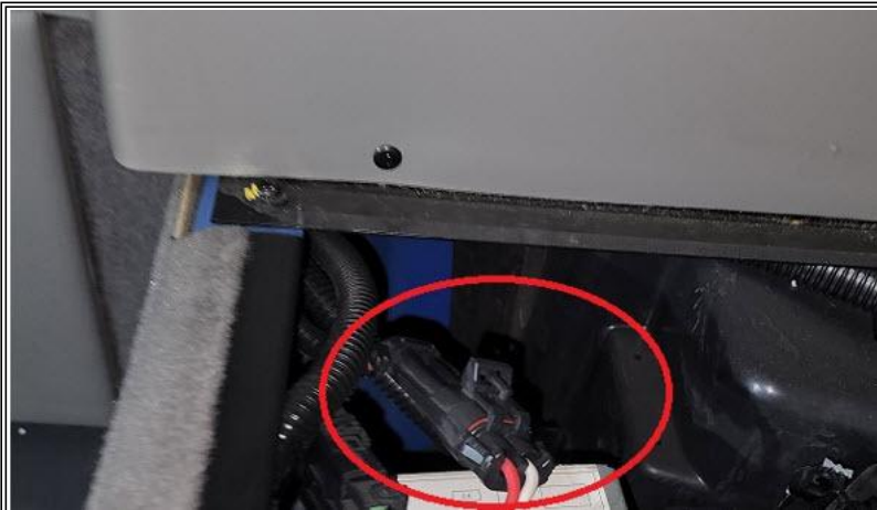
Figure 2: 100B/C No-Idle System controller power sense/ground connector
