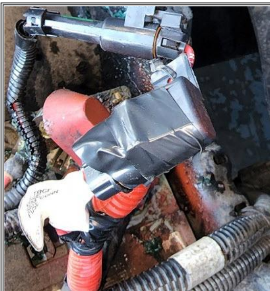
Figure 13: Fuse Holder - Fuse Removed, Cap Taped with Electrical Tape
