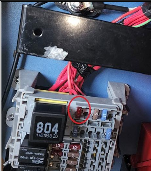
Figure 11: Assembled Sleeper PDM - 10 amp Fuse Installed in H2-E
