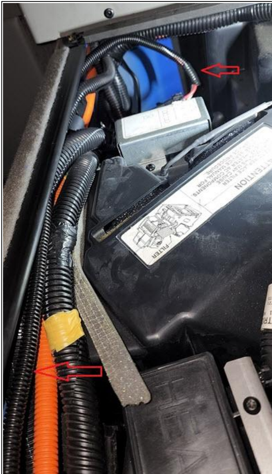
Figure 4: Routing of the 100B/C No-Idle System controller power sense/ground connector overlay
