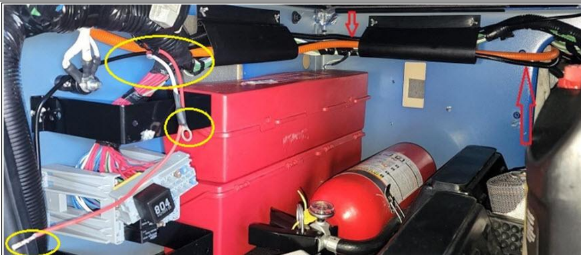
Figure 6: Routing of the 100B/C No-Idle System controller power/sense and ground connector overlay
