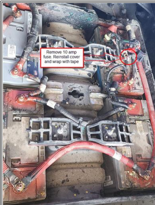
Figure 12: Auxiliary Battery Box - Fuse Removal
