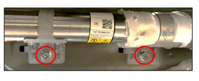
**NOTE:** Muting the noise by pressing the bracketing with you finger can be useful when confirming the rattle-type sound source.
