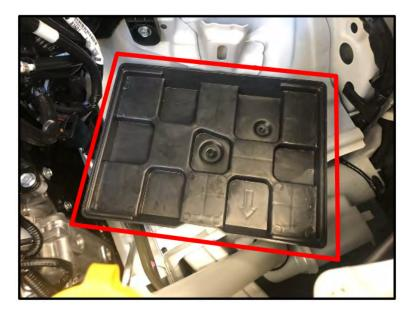
STEP 3: Replace the battery tray with the new part (p.n. 82190AN000).
