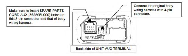
**STEP 3:** Install the new auxiliary USB terminal and adapter per the applicable Service Manual. Refer to STIS: Body & Electrical/WIRING SYSTEM > External Connection Terminal
