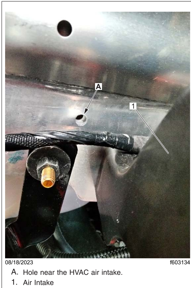
Fig. 6, Misaligned Hole Located near the Air Intake
