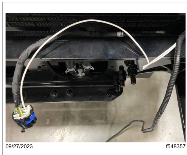
Fig. 89, Wires Trimmed to Length as Needed Prior to Splicing
