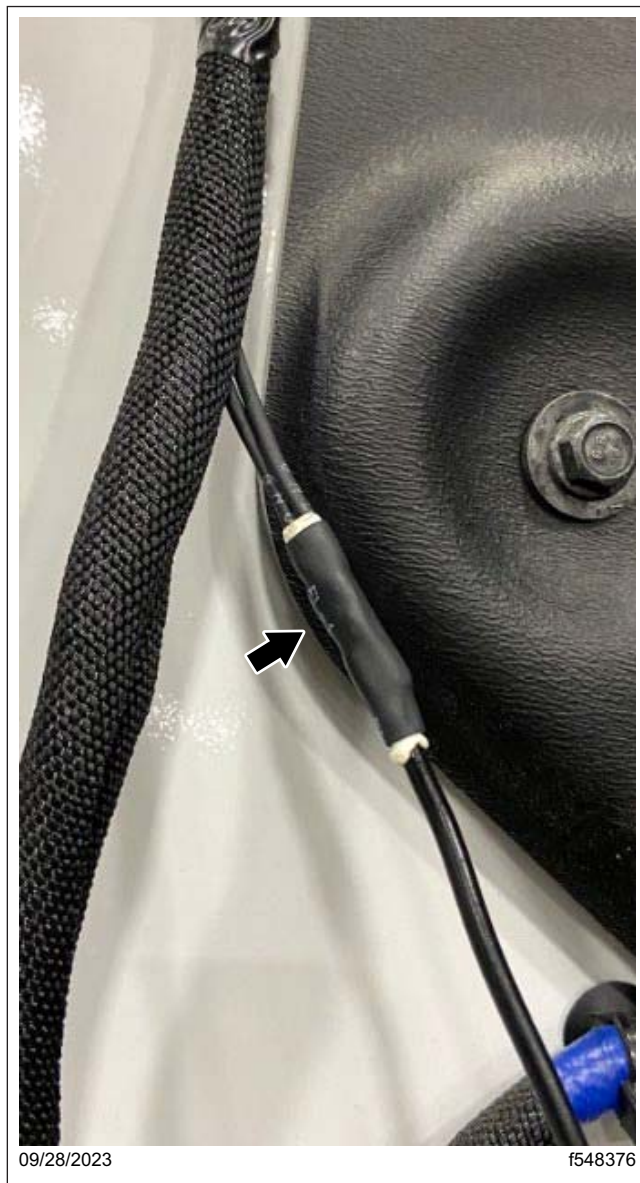
Fig. 108, Splicing the Black Wire(s) from the Marker Light to the Black Wire from the Harness (TSU CT44FRT035)
