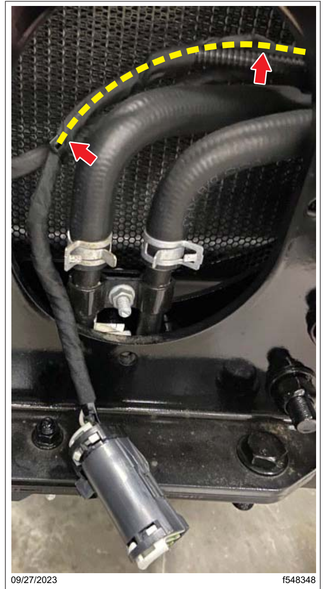
Fig. 80, Harness Path to the Plow Connectors (single connector configuration shown)
