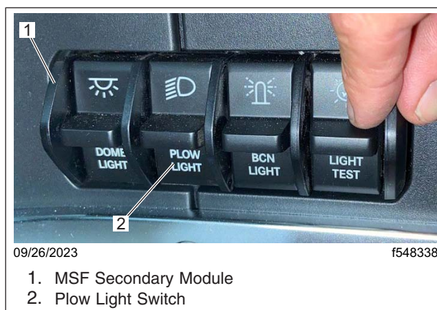
Fig. 70, Plow Light Switch in MSF Secondary Module
