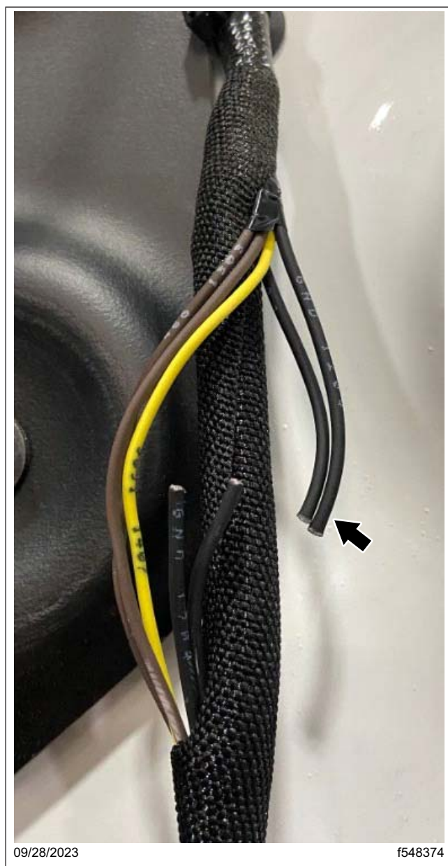
Fig. 106, Black Wire(s) Leading to the Driver-Side Marker Cut
