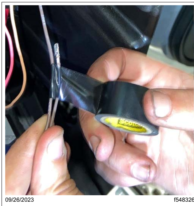
Fig. 58, Taping Up the Brown Wire
