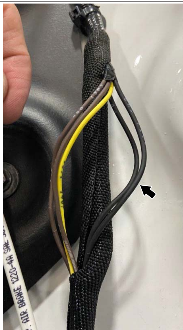
Fig. 104, Location to Expose the Wiring in the Existing Marker Light Harness (driver's side)
