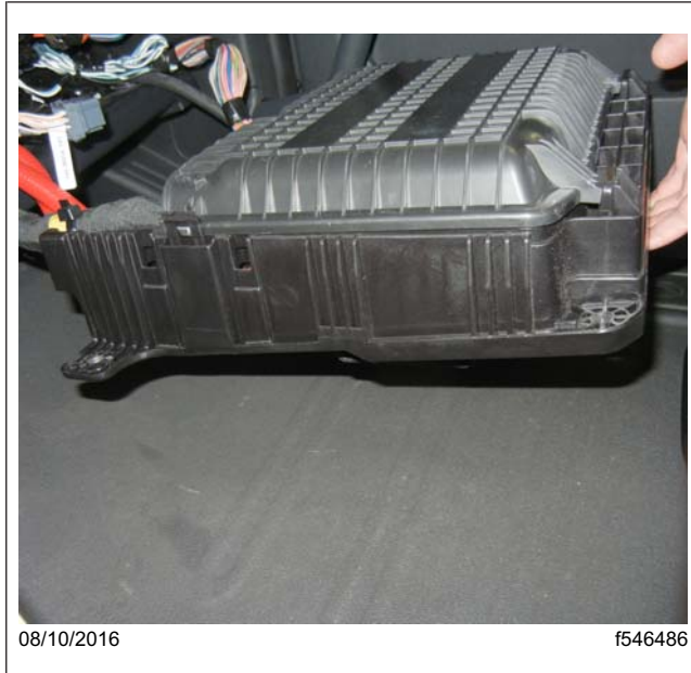
Fig. 12, VPDM Lowered to the Floor
