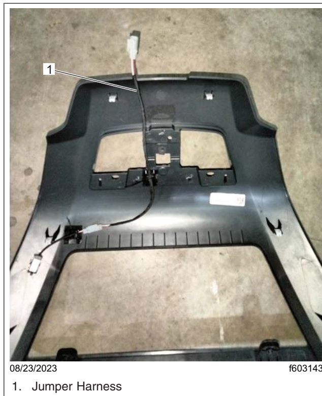
Fig. 7, Installation of the Jumper Harness
