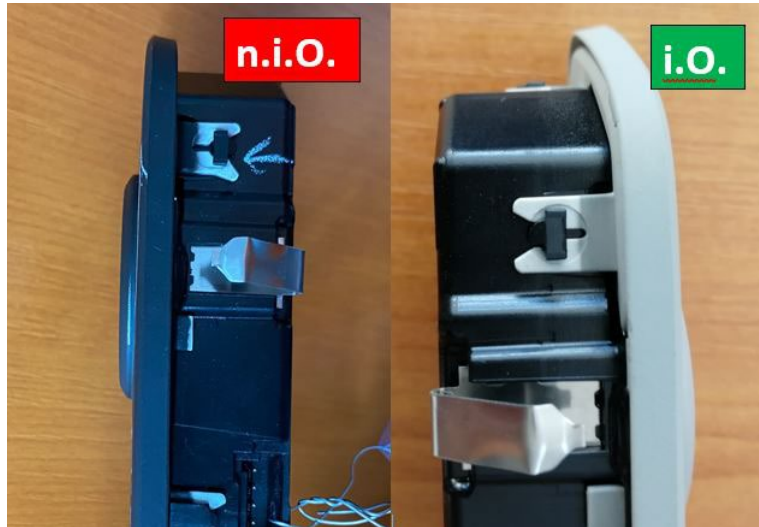
Figure 1. Left photo shows trim dislodged from base. Right photo shows trim properly seated to switch base.
