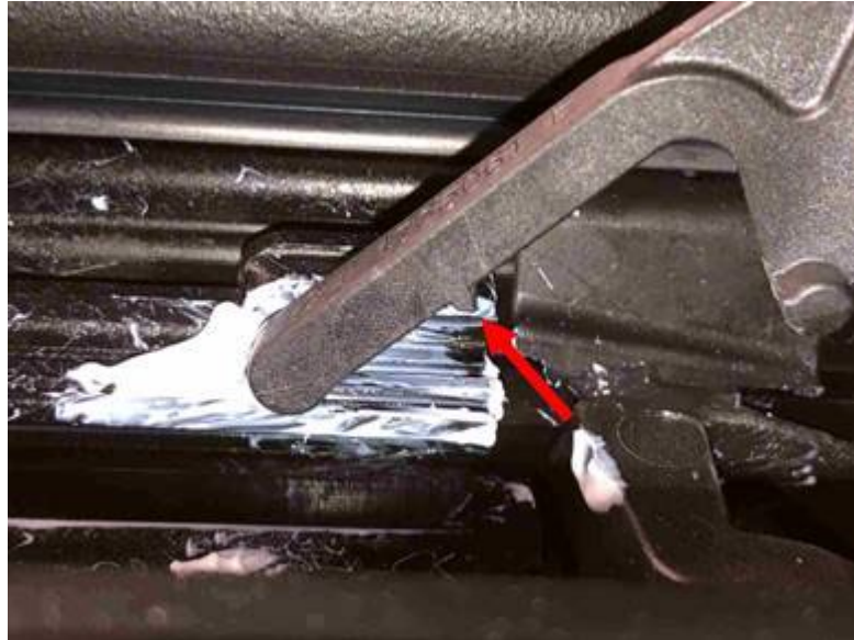
Figure 10. Tabs cast into the redesigned wind deflector.
