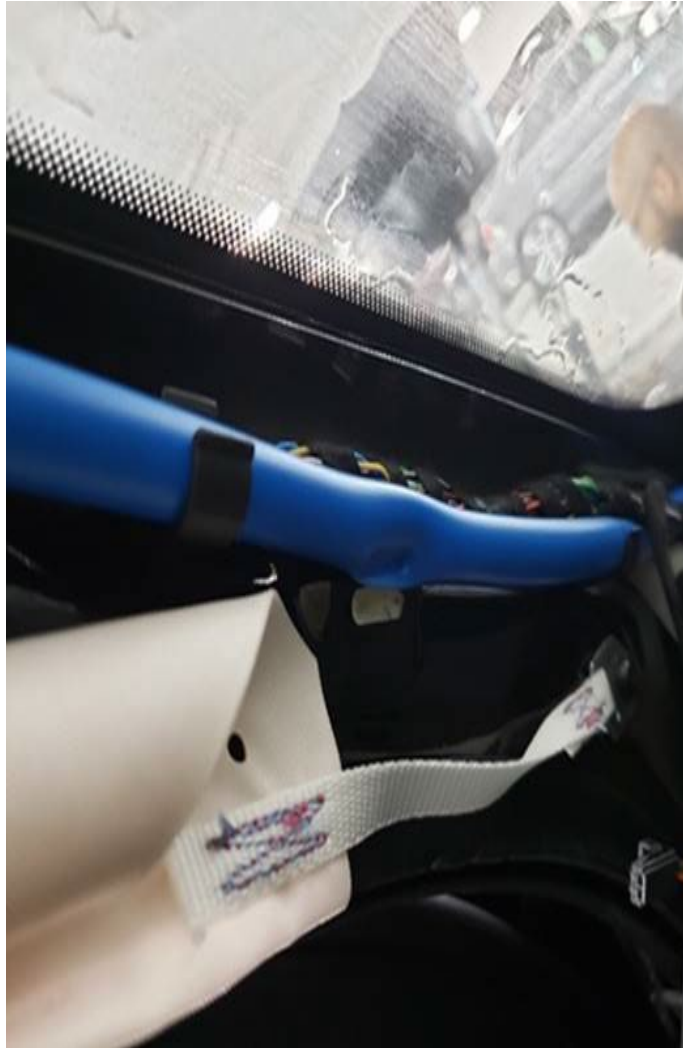
Figure 3. Sunroof drain hose pinched by the pillar trim.
