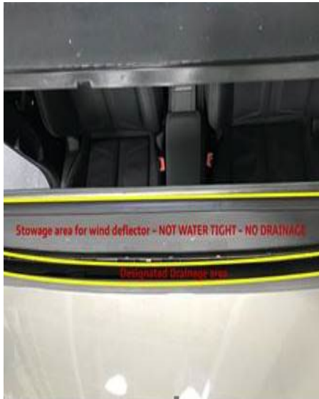
Figure 7. Areas of sunroof opening water elimination capabilities.
