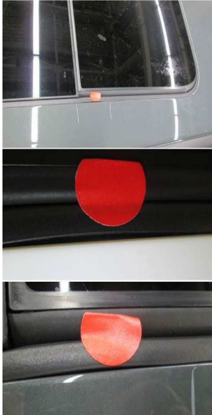
Figure 4. Detached and malformed roof opening seal.
