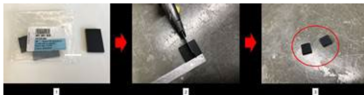
Figure 16. Preparing 2 – 10mm x 10mm pads of 251 201 525 packing.
