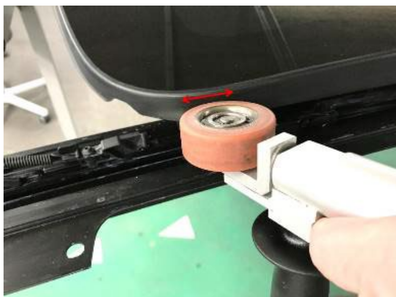
Figure 18. Applying pressure to bonded area with 3356 roller (or equivalent).
