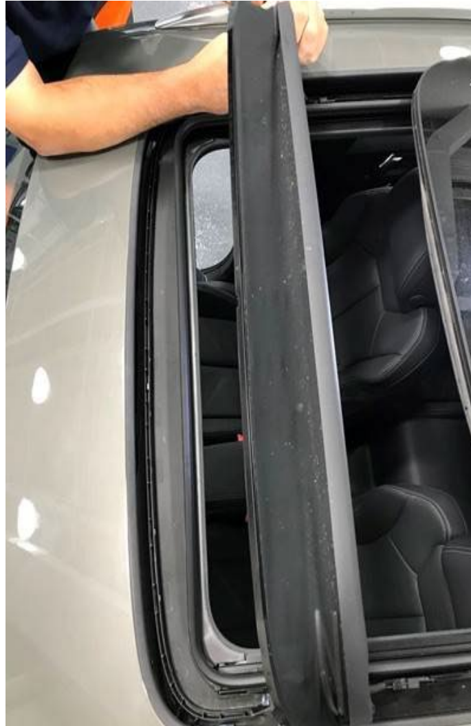
Figure 6. Front sunroof opening with the drainage exposed.
