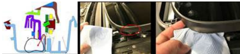
Figure 14. Area of glass panel 'skirt' to be cleaned and dried.
