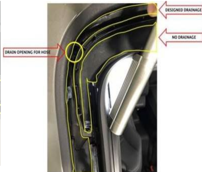
Figure 8. Sunroof water channeling diagram.
