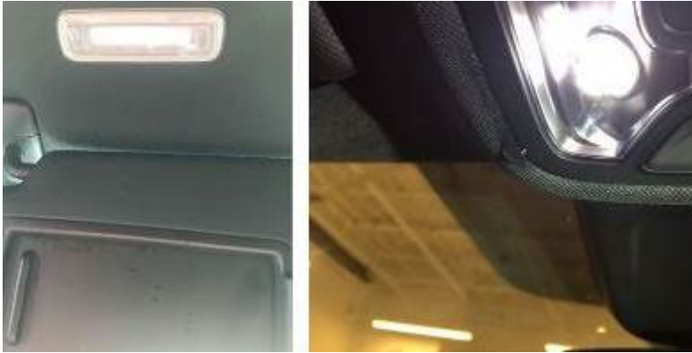
Figure 1. Water intrusion near the headliner.
