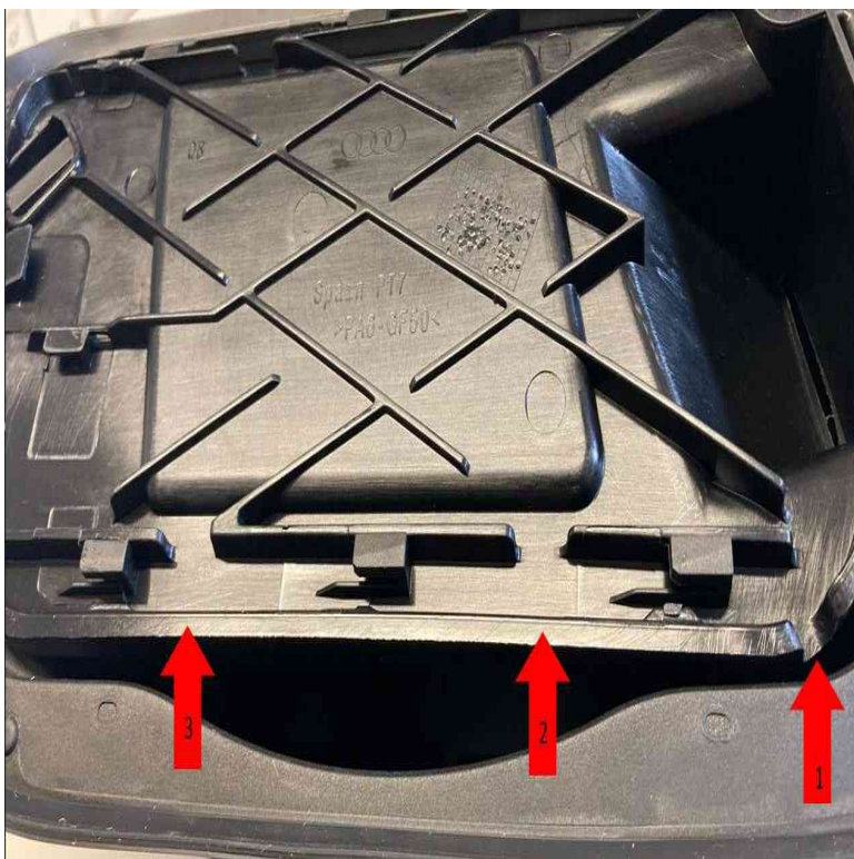
Figure 1. Adding two water drains in positions #2 & #3.
