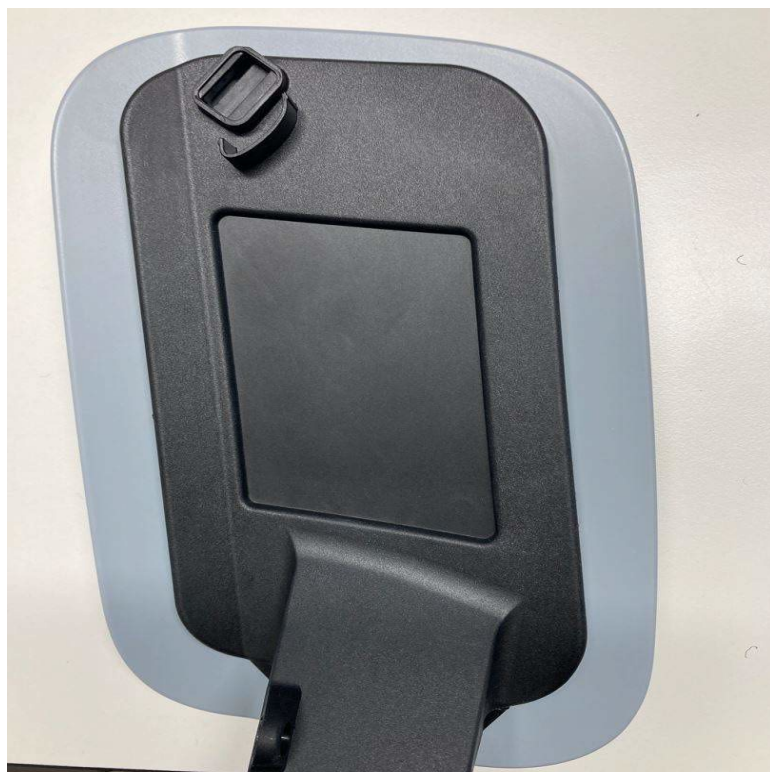
Figure 7. Original fuel filler door installed with excess adhesive removed.
