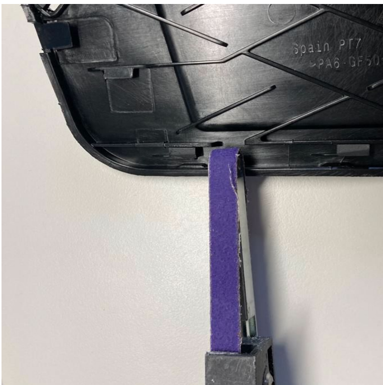
Figure 2. Use a belt sander to make additional drains.
