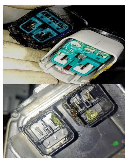
Examples of factory applied dielectric grease. Do not add to or remove the grease.
