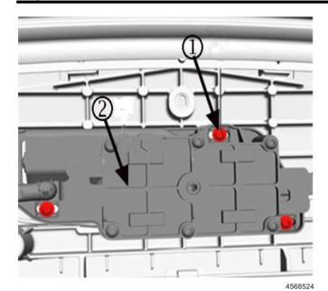
2. Loosen the three bolts (1) retaining the folding top front latch actuator motor. Refer to *Folding Top Front Latch Actuator Motor Replacement* in SI. Ensure the motor bolts are loose enough that the motor (2) can be moved freely side to side.
