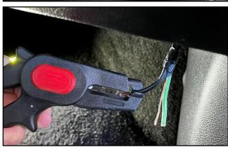
5. Cut the three (3) wires from the  $\underline{\text{new}}$  harness  $2 \frac{1}{2}$  above the connector.
