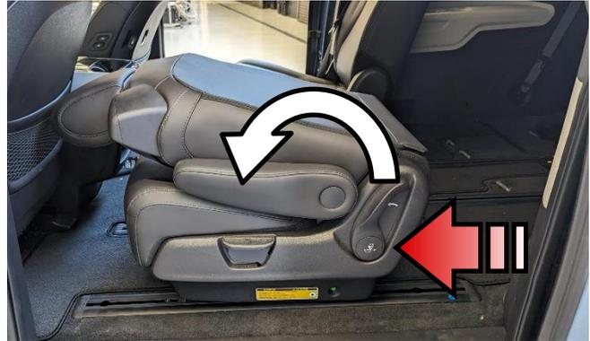
3. Remove the left side 2<sup>nd</sup> row seat by pulling the seat lock release lever located underneath the rear of the seat.
