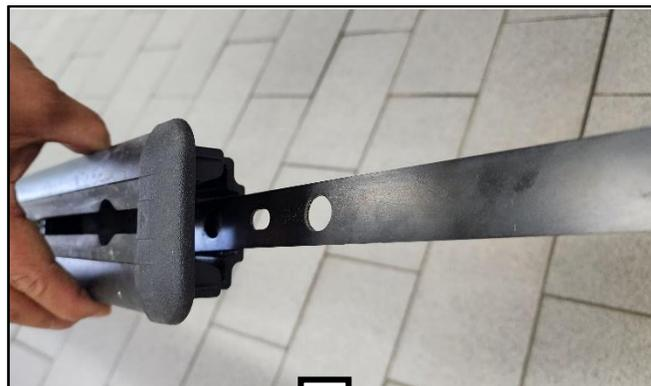
7. Re-install the outer seat rail with the inserted reinforcement plate using two (2) of the bolts removed and two (2) of the four new bolts supplied.
