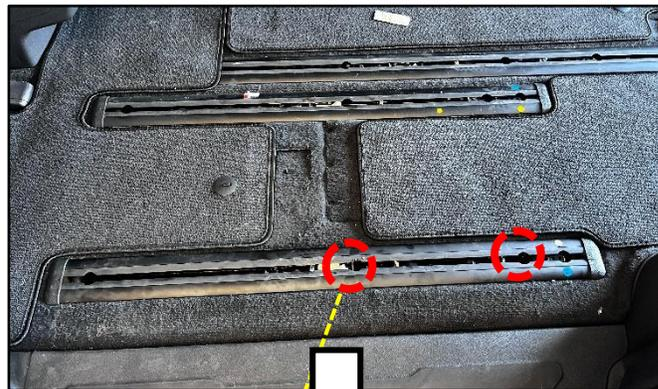
5. To access the center seat rail retaining bolt, press the seat rail lock lever downward using one hand while holding/sliding the rail with assistance from the other hand.
