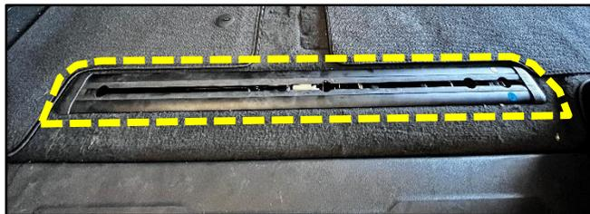
6. Insert the reinforcement plate into the seat rail as shown
