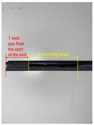
Reinstall the seal following the repair instructions listed in ISTA/AIR 54 013 052.
