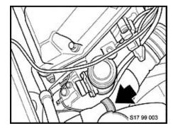
4. If the inner fabric webbing of the hose is not visible in the contact area install a protective sleeve part number 11 53 7 505 832 on the hose in the contact area.
