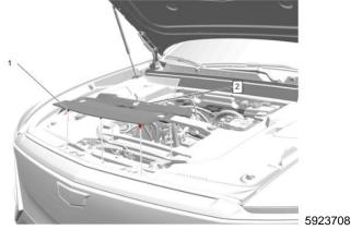
16. Install the Front Compartment Front and Side Sight Shields. Follow the steps in *Front Compartment Front Sight Shield Replacement* in SI.
