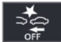
PCS warning light
