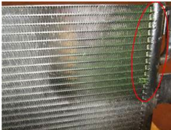
Figure 2. Evidence of a refrigerant leak at the condenser using contrast agent as the diagnostic medium.
