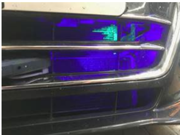
Figure 2. Evidence of a refrigerant leak at the condenser using contrast agent as the diagnostic medium.
