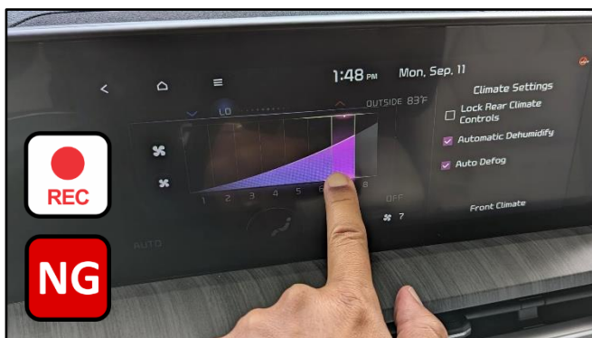
Fan blower does not set to desired speed/reverts to old setting.
