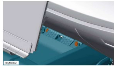
17. Remove M6x20 bolts (x2) securing floor console assembly to vehicle. Torque 5 Nm.
