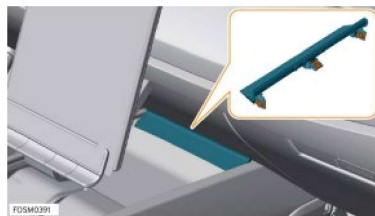
15. Release clips (x3) securing front screw cover to floor console assembly.
