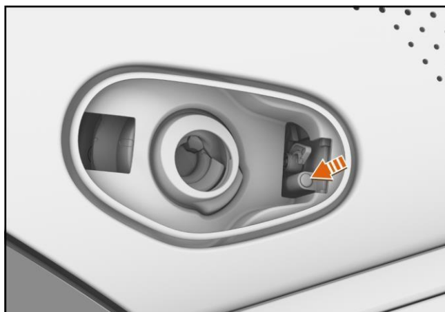
Image 2 Filler Flap Actuator Shaft
