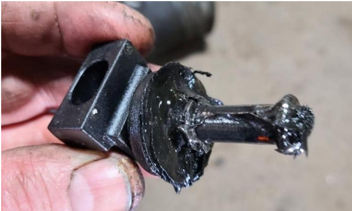
Figure 1 - Melted Speed Sensor
