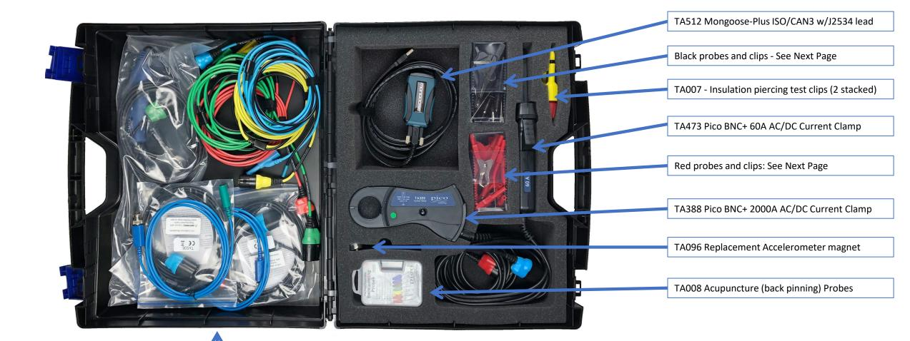
TA398 Pico BNC+ Coil on Plug/Signal probe TA404 PicoBNC+ Test Lead: 4mm permanent ground, 3m Blue TA405 PicoBNC+ Test Lead: 4mm permanent ground 3m, Red TA406 PicoBNC+ Test Lead: 4mm permanent ground 3m, Green TA407 PicoBNC+ Test Lead: 4mm permanent ground 3m, Yellow TA329 Ultrasonic parking sensor detector TA330 Keyless entry carrier signal detector TA506 BNC+ 10:1 Attenuating Test Lead (2)
