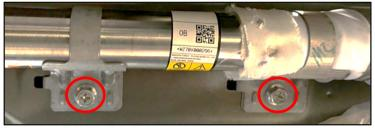
**NOTE:** Muting the noise by pressing the bracketing with you finger can be useful when confirming the rattle-type sound source.
