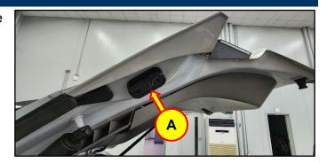
2. Remove the mounting screws and remove the tailgate guide bumper (A).
