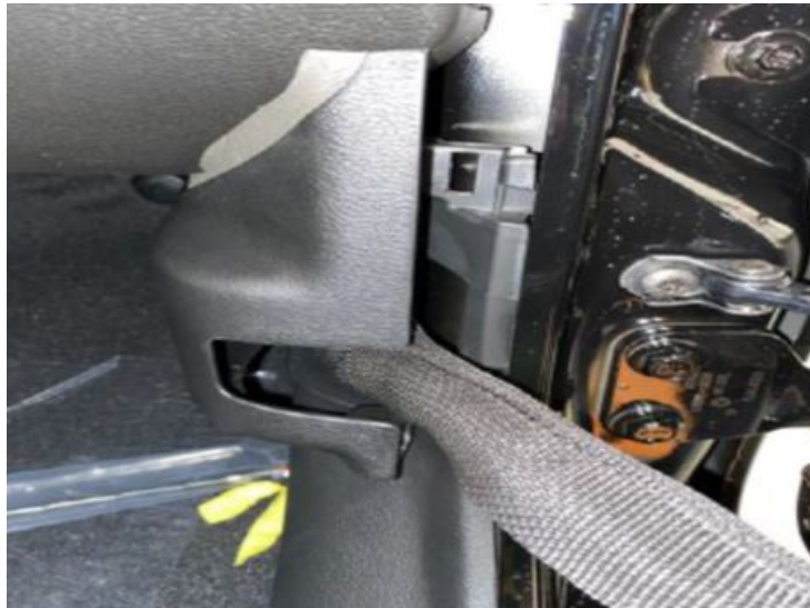
Fig. 1 Trim Panel Not Properly Seated
