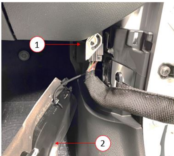
Fig. 3 Wire harness Without Trim Panel
