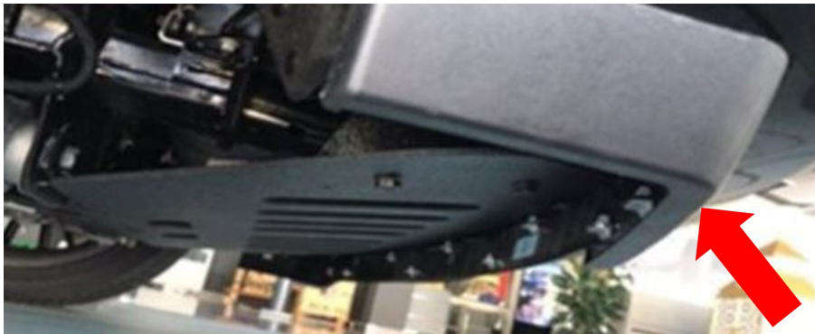
Fig. 1 Incorrect Air Dam Installed
