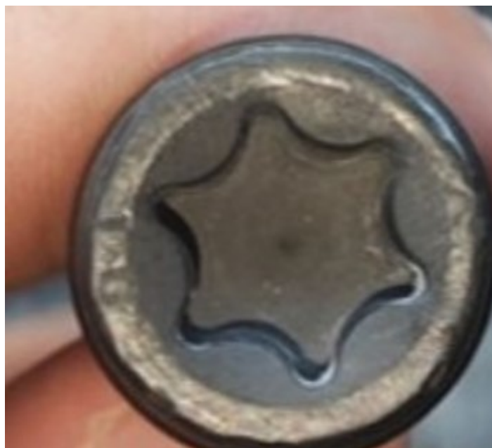
Fig. 2 Incorrect Head Fastener
