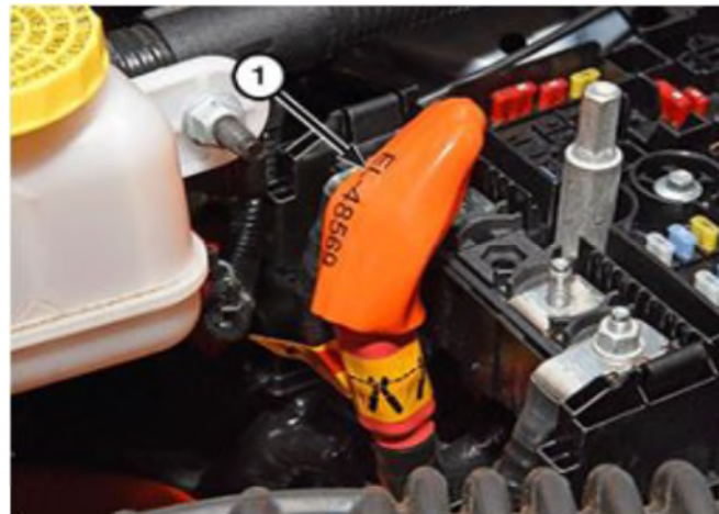
Figure 1 – 12-Volt Battery Cable
