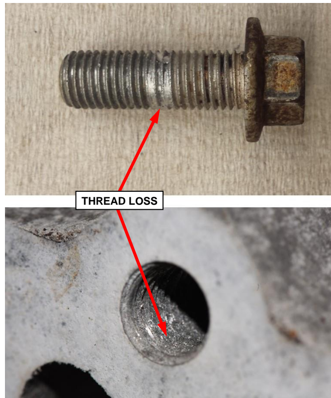
Figure 18 – Inspect for Thread Loss
