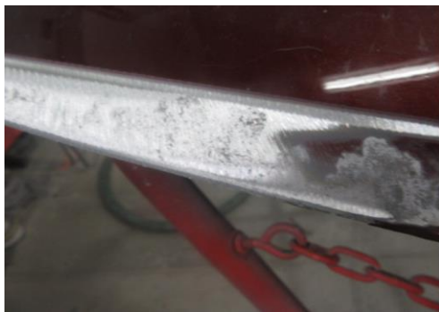
Perforation/Pitting Found After Sanding Examples (Fig. 1)
