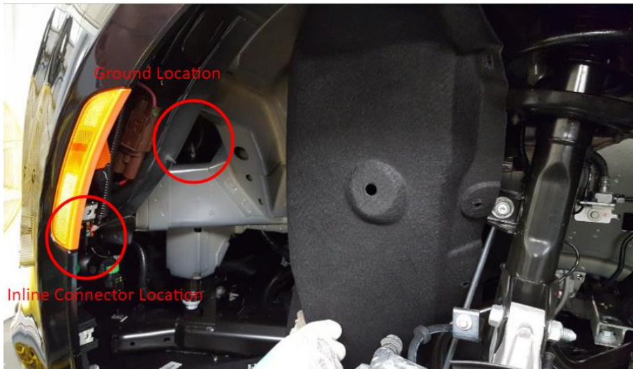
Ground and Inline Locations
