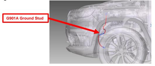
Repair: If the G901 attachment to the frame is loose, tighten the ground to 13 Ft. Lbs.
