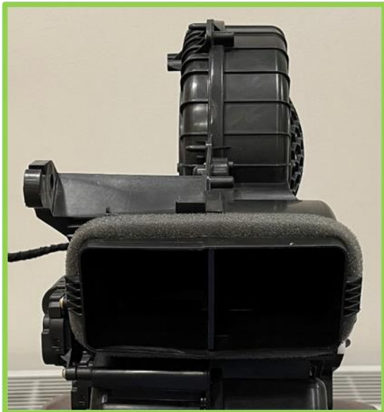
Correct HVAC Module Outlet Seal
