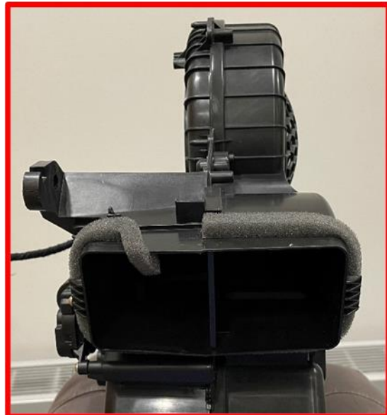
Incorrect HVAC Module Outlet Seal
